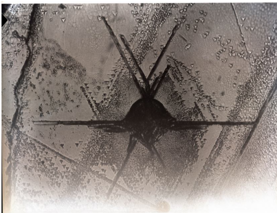
Fig. 4. Etchpit rows along the Pin indentation mark
