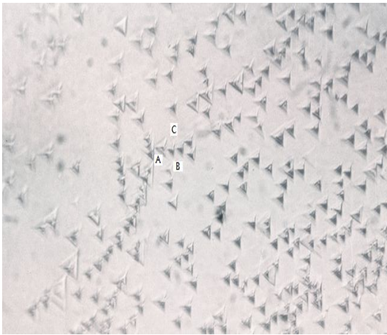
Fig. 3. Low angle boundary and etchpits on the crystals.
