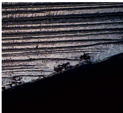
Fig. 1. Parallel Striation with equidistance observed on the top free surface of the crystals
